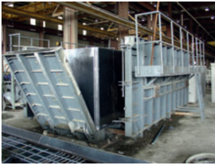
Figs. 5, 6 and 7: De-moulding process without need of removing parts from inner core by Toyotaforms
